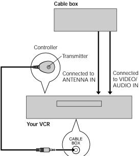
This procedure is required if you receive your TV channels through a cable box (descrambler). The Controller allows the VCR to automatically switch the cable box channel during timer-recording. The Controller is effective for recording shows that have been programmed using G-CODE ( $\square$  pg. 40) or On-Screen Timer Programming ( $\square$  pg. 42).
