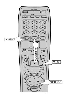
Insert editing replaces part of the recorded scene with new material. Both the picture and Hi-Fi audio soundtrack are replaced with new ones, while the normal audio soundtrack remains unchanged. If you wish to change the normal audio track as well, use the audio dubbing function simultaneously. Use your VCR as the recorder.
