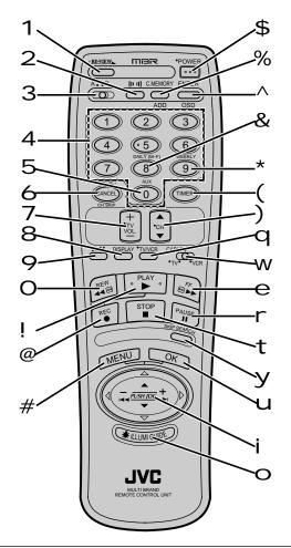
Buttons with a small dot on the left side of the name can also be used to operate your TV: POWER, TV VOL. +/-, CH ▲▼, TV/VCR. Use these buttons with the TV/CABLE/VCR switch set to "TV".
