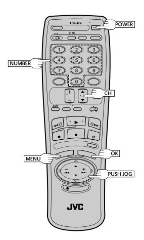
The G-Code timer programming system eliminates the need to input channel, date, start and stop time data when setting the timer record function. Simply key in the G-Code number for the TV program you wish to record (found in most TV listings) and the VCR's timer is automatically programmed.
